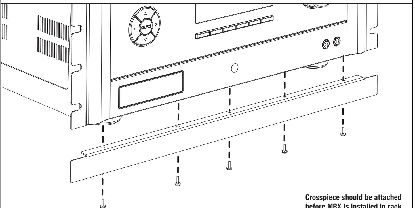
Crosspiece should be attached before MRX is installed in rack.
